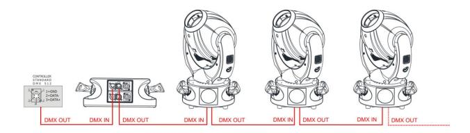
For Installations where long distance DMX cable connections are needed, we suggest to use a DMX terminator.
