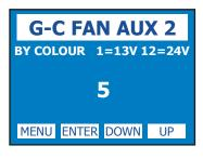
GOBO-COL. FAN SPEED WHEN COLOUR WHEEL INSERTED
