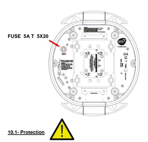
The use of a thermal magnetic circuit breaker is recommended for each RAPTOR. A good earth connection is essential for the correct operation of the projector.
