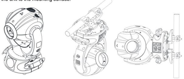
The supporting structure from which the unit is hung should be capable of bearing the weight of the unit, as should any clamps used to hang it.
