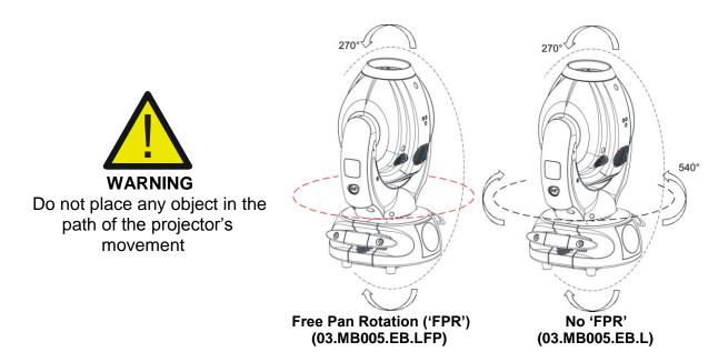
Please Note: If two different RAPTOR model (with and without FPR) are controlled at the same time via DMX controller, be shure that channel 6 (PAN FAR) is set to value 0. In this way, the RAPTOR with FPR will react to DMX same as RAPTOR with no FPR function.
