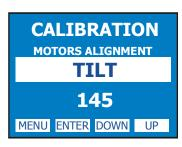
TILT ALIGNMENT To align Tilt position
