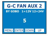
GOBO-COL. FAN SPEED WHEN GOBO WHEEL INSERTED
