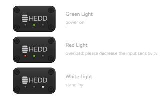
The monitors automatically jump into stand-by after 30 minutes. They wake back up when audio is played.
