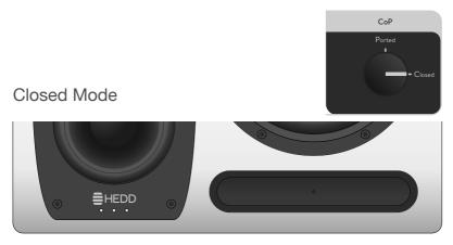
In closed mode the HEDD MK2 speaker functions as an infinite baffle speaker. This results in a cleaner sound and increased resolution. However, a 6-10 dB reduction in maximum sound pressure level (depending on the audio material) for low frequencies is the consequence.
