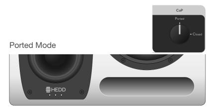
This is the default operating mode. The bass reflex ports are open and allow for a powerful low-end reproduction. This operation mode allows for a higher efficiency and while maintaining access to lower bass regions.
