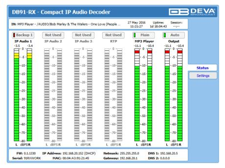
The main Status window contains information on the device's current status - the LED bar-graph representation of the audio sources. The interactive buttons placed over the LED bar-graphs allow the audio source to be manually changed.
