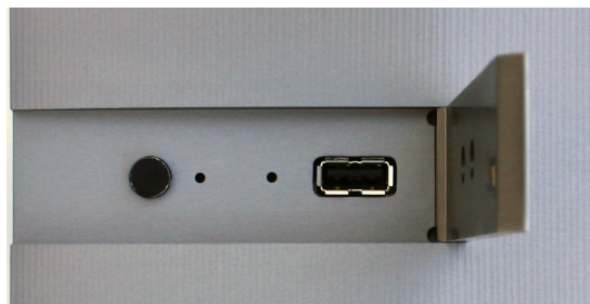
Figure 2: Power Button Door, open position
