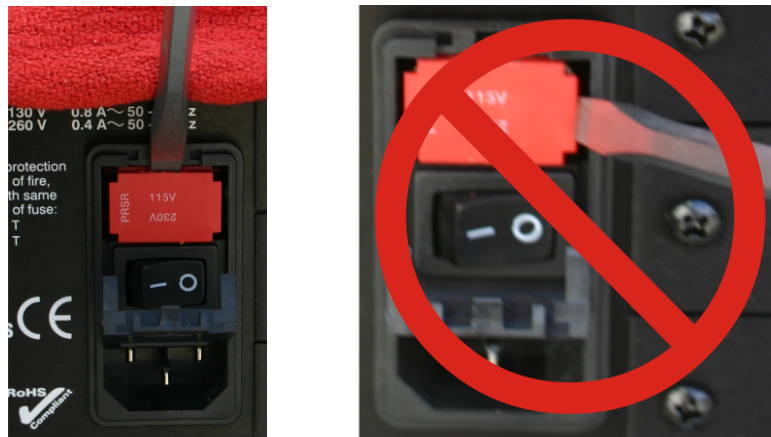
Figure 14. Accessing Fuse Block. Pry from top or bottom only.
