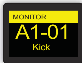
Monitor screen showing the first input of the input card in slot A
