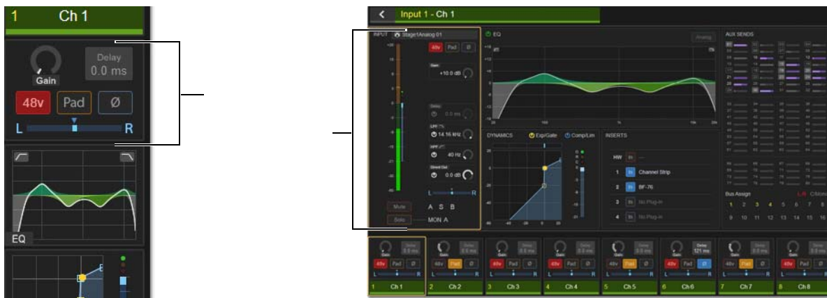
Input touch zone on the CTM in Meters view (left) and in Channel view (right)
