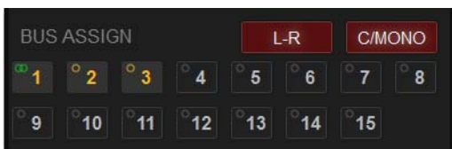
Bus Assign section showing a channel assigned to Mains L-R, C/Mono, and Groups 1, 2, and 3
