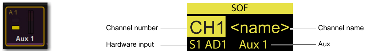
A Channel Tile showing a soloed Aux (left) and a channel display indicating Sends on Faders mode (right)
