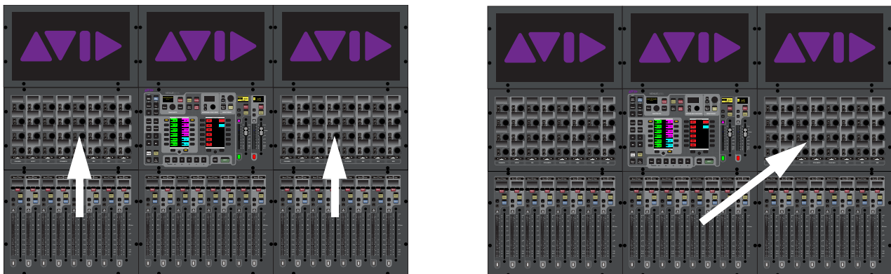
Selecting a channel below a CKM (left) and below the MLM (right)
