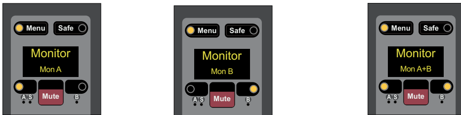
A channel display showing a channel routed to Monitor Bus A (Left) Bus B (center) and Buses A and B (right)
