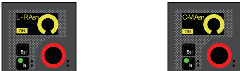
Encoder and display showing a channel assigned to Mains L-R (left) and C/Mono (right)
