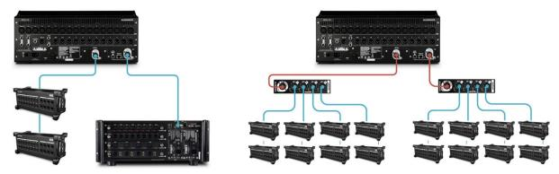
① SQ does not support DX redundancy.
