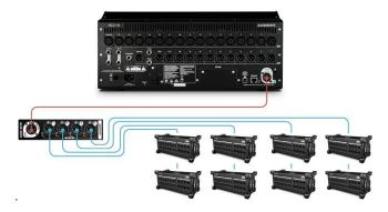
An optional SLink I/O module can be installed in the SQ I/O port to allow further DX connectivity.
