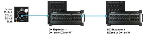
Any combination of two DX168/DX164-W expanders is supported per socket in Cascade mode with all inputs and outputs accessible to the mix engine.
