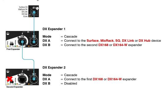
Please refer to the table below for channel mapping when using DX Expanders in Cascade mode.
